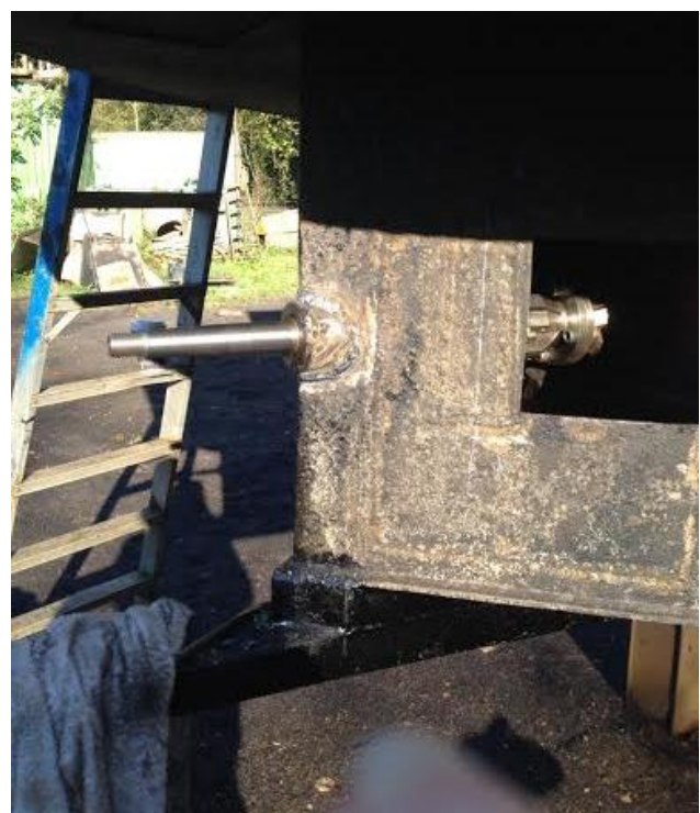
New propeller shaft in place
